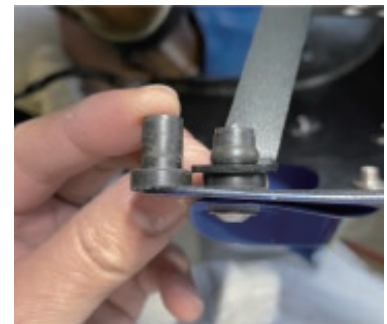
Comparison with New Well Nuts
